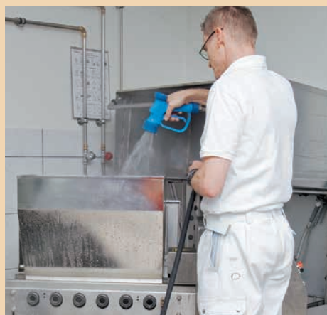
Cleaning the hopper with water
