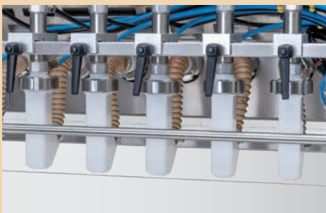
Final cut-off device for viscous fillings and cut-off wire system for fibrous fillings
