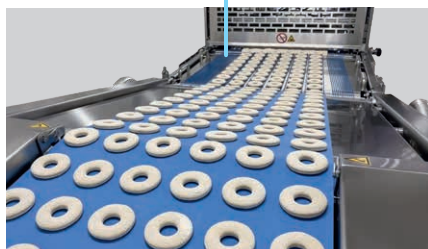
5 Reliable panning of the dough pieces in the proofing cabinet
