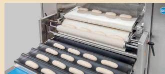
The RONDO long-moulding units automatically and reliably manufacture sandwich rolls and mini baguettes from dough pieces.
