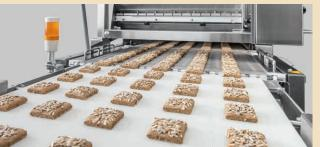
Refine your rolls with grains and seeds. RONDO depositors for coarse materials can sprinkle seeds on the top and underside of your rolls.
