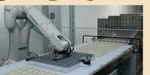
With the unique RONDObot you can mould artisanal style bread and rolls with an open crumb structure. These can be produced from highly hydrated doughs with a water content of over 80 % and a resting time of up to two hours.
