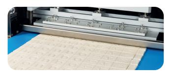
The dough sheet can be stamped into a wide variety of shapes. Stamps can be custom-made according to your request.
