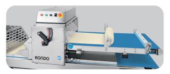
In sheet cake production, the baking sheets are placed on the conveyor belt of the make-up line ...
