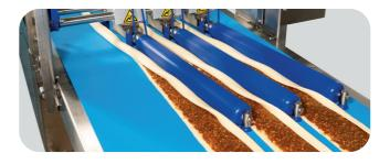
For smaller rolled pastries, a number of rolling guides are used in parallel.
