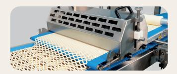
The toboggan can also be used to place a second dough sheet on top of the first one. This allows for even more possibilities in the production of special pastry.
