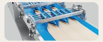
To produce palmiers, the dough sheet is cut into strips...
