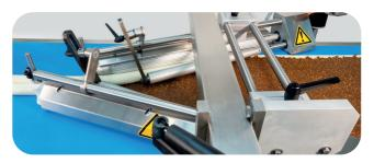
The double rolling unit enables the production of special double rolls. The dough sheet is rolled in from both sides.
