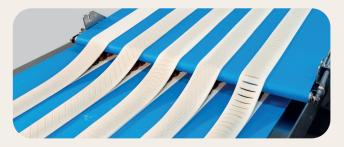
The dough sheet is cut into several strips. The filling is then placed on every other strip. Using the toboggan, each strip with filling is covered with a strip of dough. Finally, the product is cross-cut or stamped into shape.
