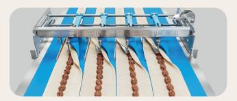
The dough sheet is folded once with a single-row or multi-row folding station. It is then cut to the desired length...
