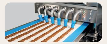
Continuously, discontinuously or in spots – fillings ranging from soft and creamy to solid are placed on the dough sheet in one to six rows.
