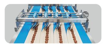
The dough sheet is folded twice with a single-row or multirow folding station. The closing fold is on top or underneath the final product according to your wishes.
